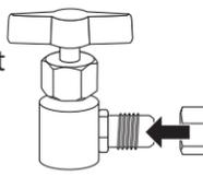
2. Open valve to coat the inside of the cap, then close the valve.
